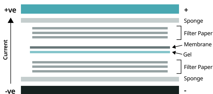
Figure 7. A schematic representation of protein transfer from the gel to a membrane. Negatively charged proteins move up towards the positive cathode and onto the membrane.
